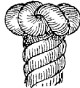
FIG. 114.—Wall knot.
