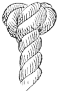
FIG. 122.—Double crown (complete).
