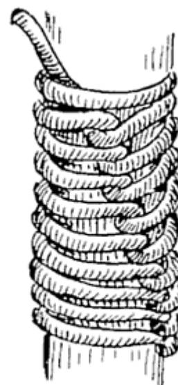
FIG. 140.—Half-hitch work.
