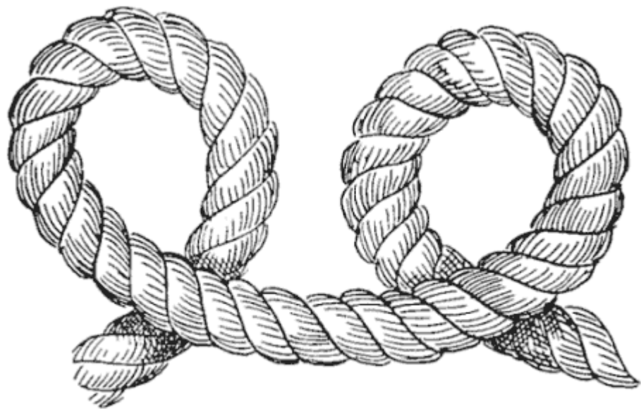
FIG. 5.—Cuckolds' necks.
