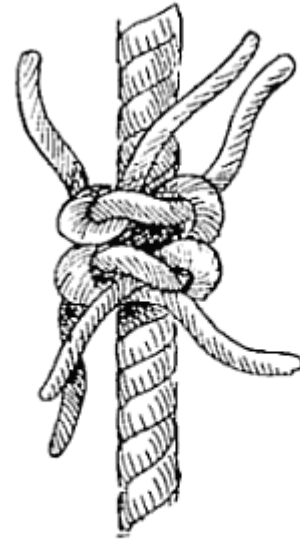
FIG. 118.—Shroud knot (making).
