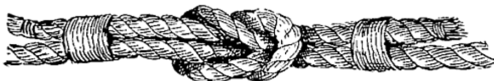
FIG. 15.—Square knot with ends seized.
