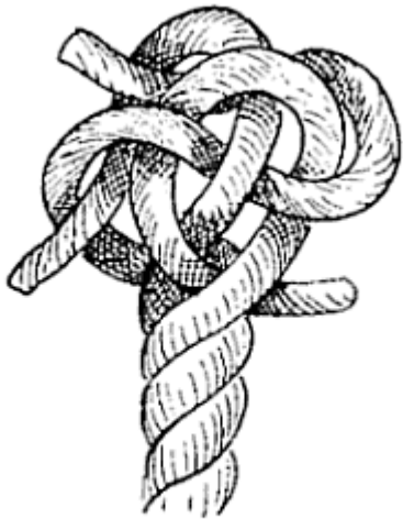
FIG. 121 A .—Making double crown.
