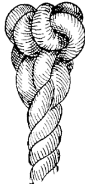
FIG. 115.—Wall knot (making).
