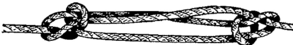
FIG. 82.—Sheepshank for free-ended rope.
