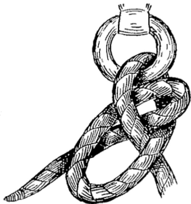
FIG. 33 —Slippery hitch (tying)
