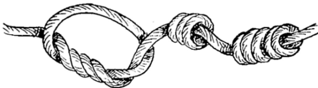
FIG. 69.—Three- and fivefold shortening.
