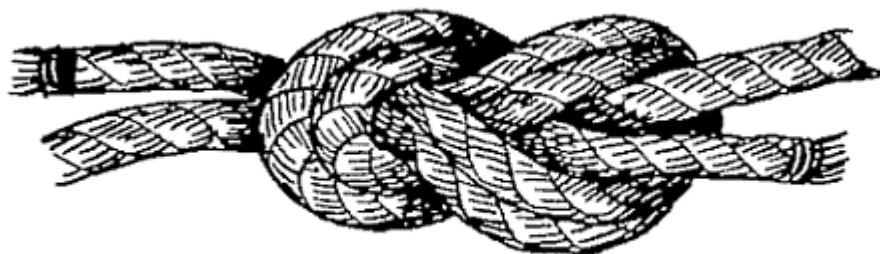
FIG. 24.—Double figure-eight knot (complete).
