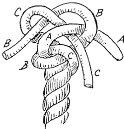
FIG. 124.—Wall crowned (making).
