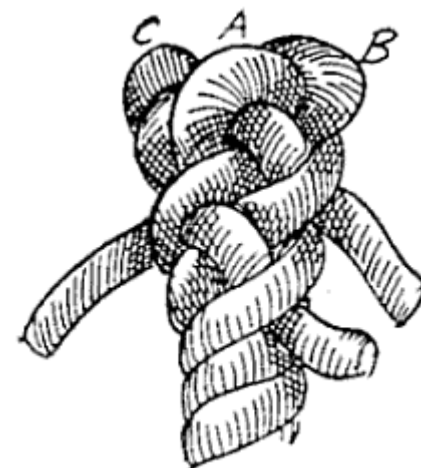
FIG. 111.—Single crown (making).
