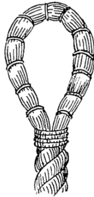
FIG. 90 B .—Flemish eye (complete).
