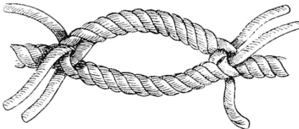
FIG. 109.—Cut splice.
