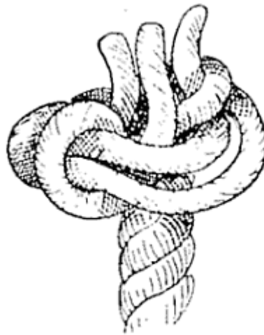
FIG. 121 B .—Making double wall.
