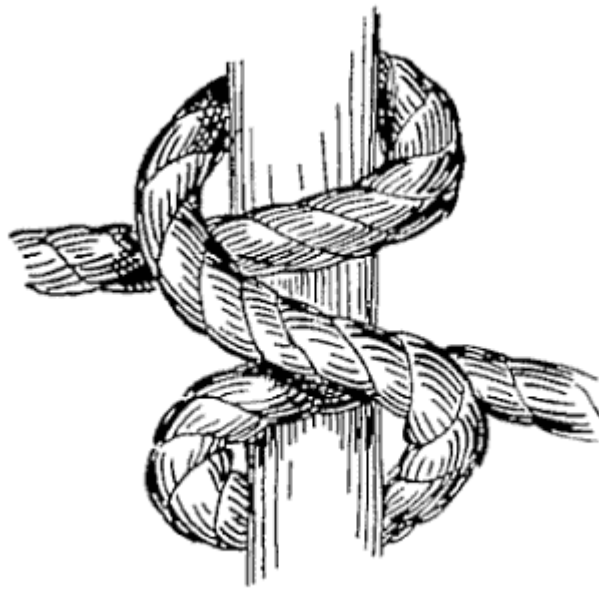
FIG. 36 A.—Clove hitch or builder's hitch (tying).
