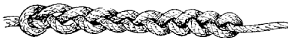
FIG. 72.—Twist braid (complete).
