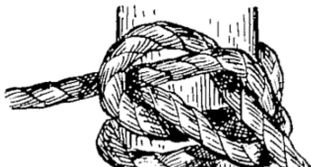
FIG. 36 A.—Clove hitch or builder's hitch (tying).
