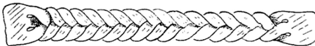
FIG. 74.—Leather braid (complete).
