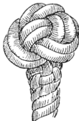
FIG. 127.—Double wall and crown (complete).
