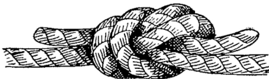
FIG. 19.—Ordinary knot (finished).
