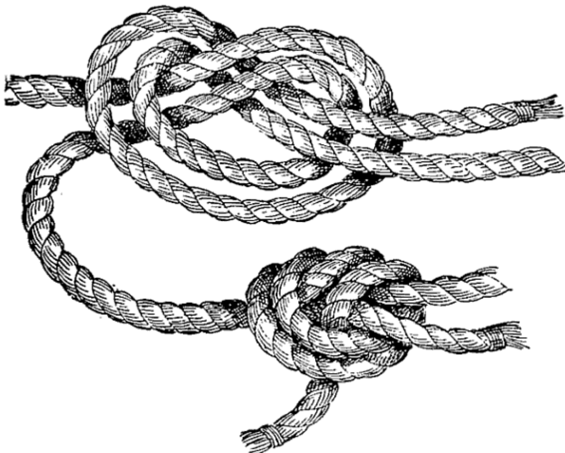
FIG. 16.—Open-hand knots.
