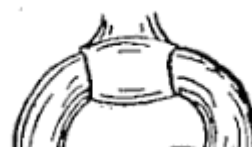
FIG. 30.—Lark's head with toggle (A).
