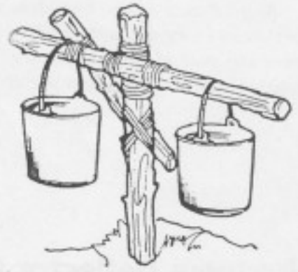
FIRE BUCKET RACK
